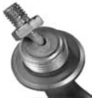
BROKEN EPOXY SEAL
