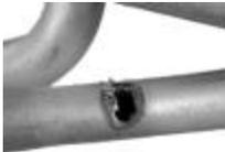
**SHEATH BURNED-OUT DUE TO DRY FIRE**
